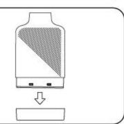
4.Remove the sticker from the contact of the pre-filled pod.
